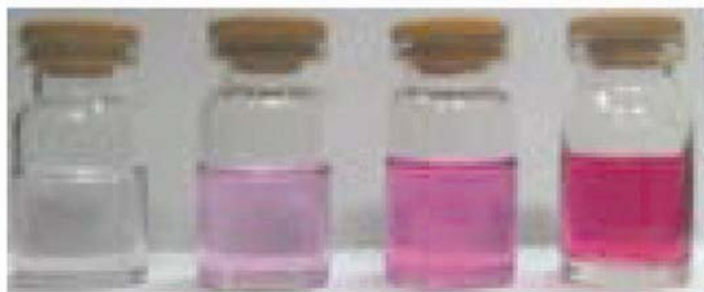
Figure 6. Photographs of RHN in \text{CH}_3\text{CN}/\text{water} ( \text{CH}_3\text{CN}:\text{H}_2\text{O} , 40 : 60, v : v, 0.04 M HAc-NaAc, pH 5.0) in the presence of different concentration of \text{Cu}^{2+} (from left to right): [\text{Cu}^{2+}] = 0, 5, 10 and 50 \mu\text{M} , respectively.
